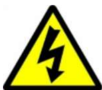
Figure 8-5: Symbol for Electrical Hazard
