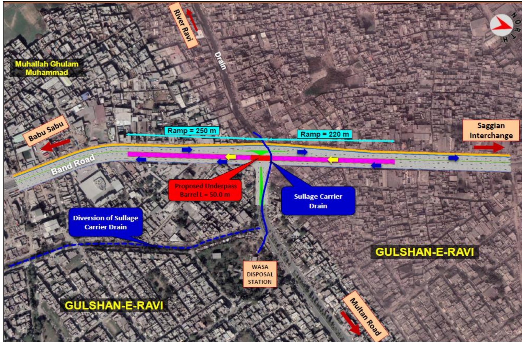
Figure 5-4 Diversion Plan for Sludge Carrier Drain
