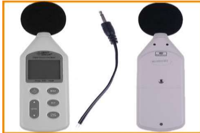
Figure 3-7: Noise Monitoring Equipment
