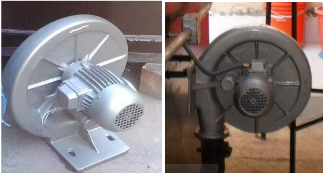
Figure 3-6: View of Air Supply Fans
