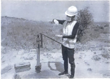
Figure 1: Ground Water Sampling
