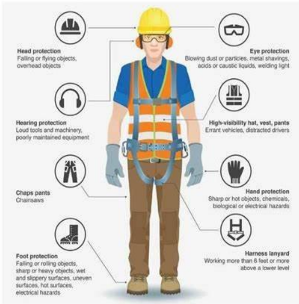
PPE for Construction Site
