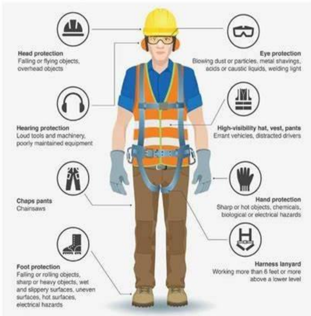
PPE for Construction Site
