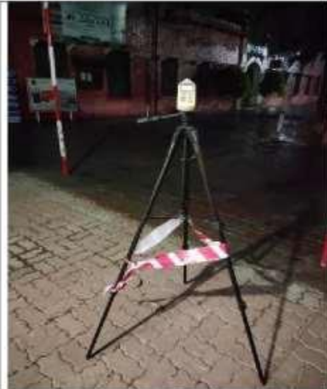
Fig9: Noise Level Monitoring night time at Government College of Technology, Sahiwal using Digital Sound Level Meter
