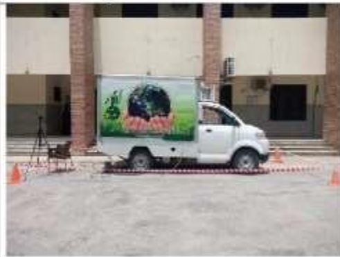
Fig7: Ambient Air Monitoring at day time at Govt. College of Technology, Bahawalpur using Mobile Ambient Air Monitoring Station
