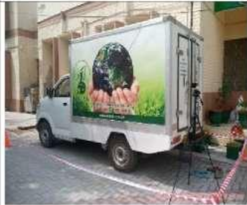
Fig12: Ambient Air Monitoring at Day time at Govt. college of Technology Women, Faisalabad using Mobile Ambient Air Monitoring Station
