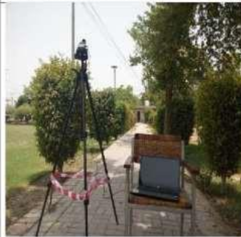
Fig11: Noise Level Monitoring day time at Government College of Technology, Bahawalpur using Digital Sound Level Meter
