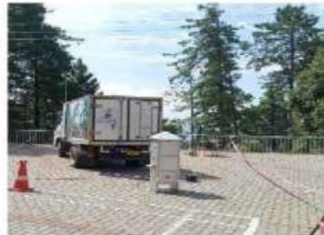
Fig4: Ambient Air Monitoring at day time at Government Staff Training College, Murree using Mobile Ambient Air Monitoring Station
