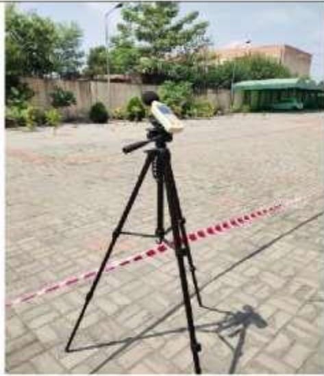
Fig10: Noise Level Monitoring day time at Government College of Technology, Gujranwala using Digital Sound Level Meter
