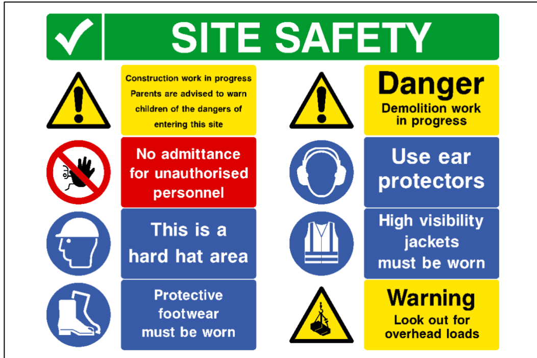
Figure 11-2: Safety signs for Constructional Phase
