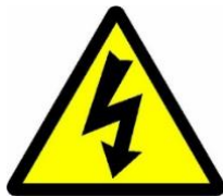
Figure 10-5: Symbol for Electrical Hazard
