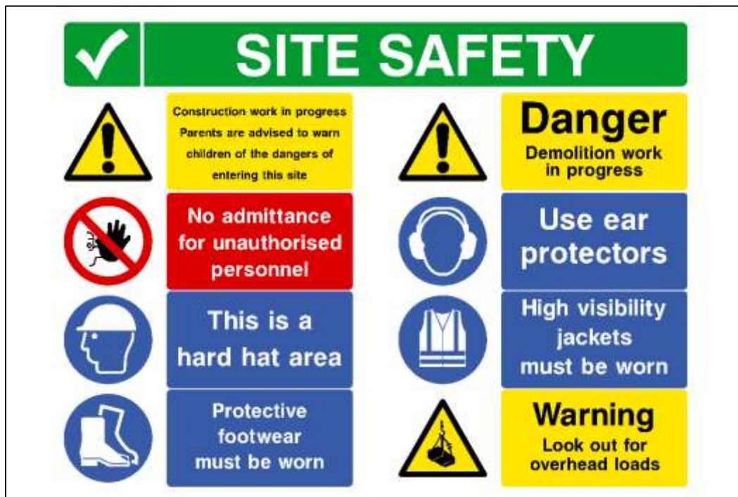
Figure 11-2 Safety signs for Constructional Phase
