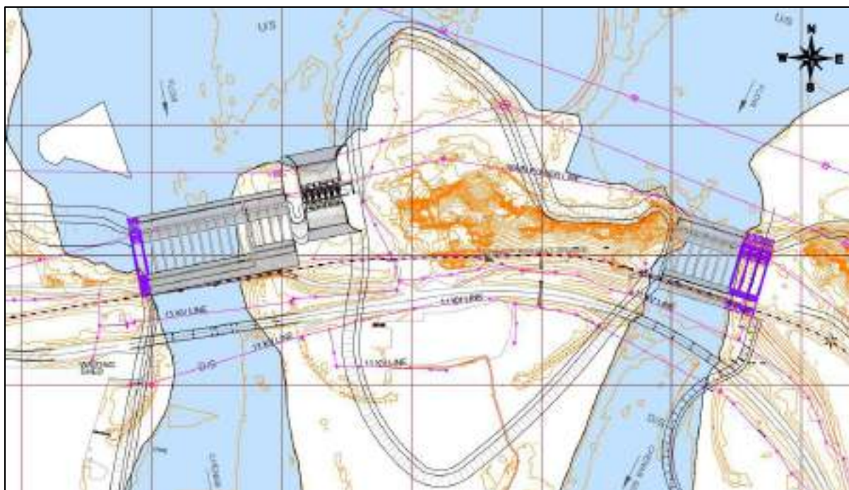
Figure 4.3: Alternative-2 Layout of Bays and Power House
