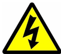
Figure 10-5 Symbol for Electrical Hazard
