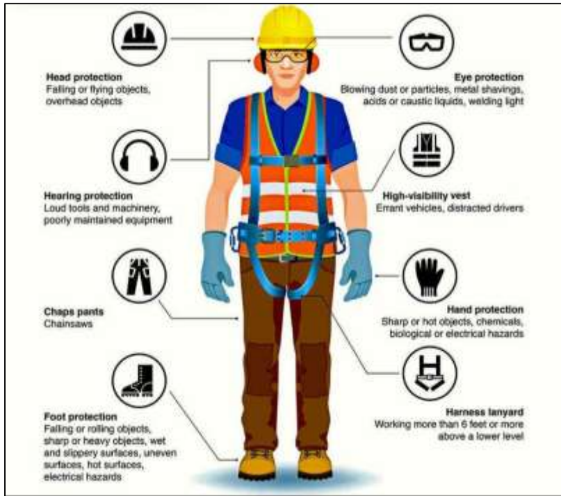
Figure 11-1 PPEs for Construction Phase
