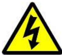
Figure 10-5 Symbol for Electrical Hazard
