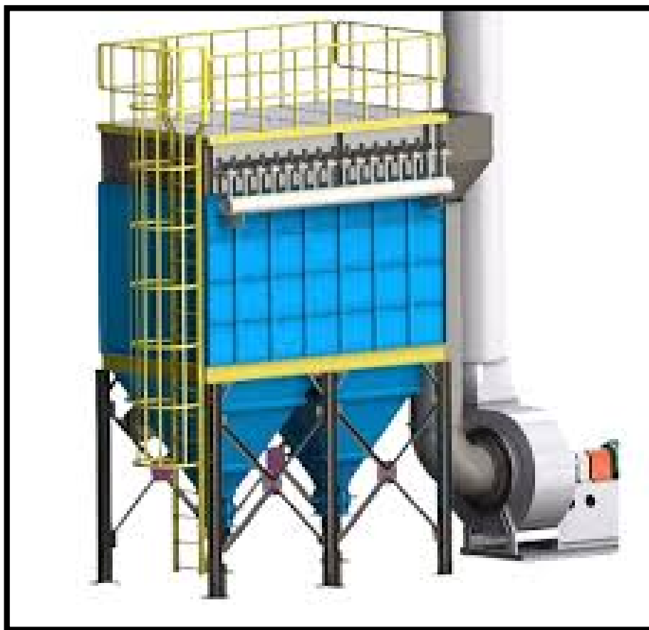
Figure 5. Indicative diagram of baghouse filters to be used for air emissions control
