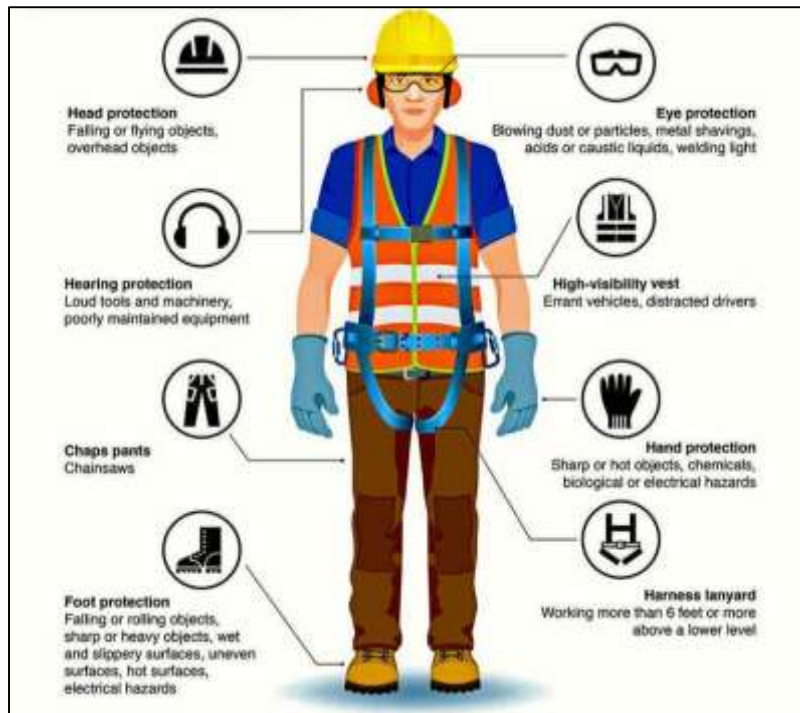
Figure 11-1 PPEs for Construction Phase
