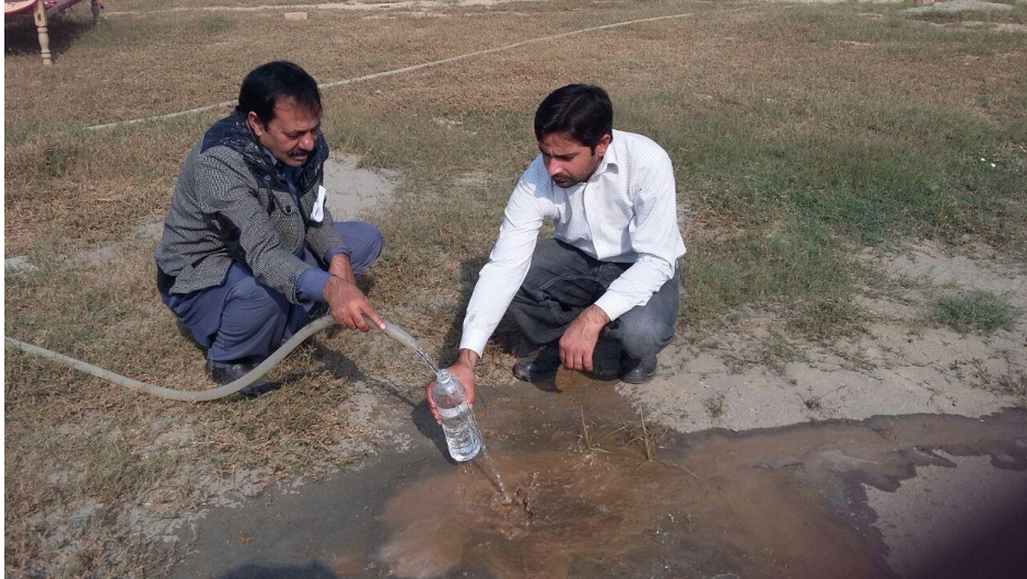
PP 3.9: Sampling of existing underground water in the area.
