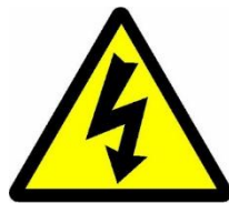
Figure 10-3: Symbol for Electrical Hazard
