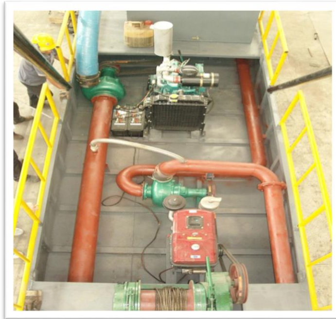
Figure 2.3 Inner structure of suction dredger
