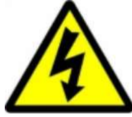
Figure 9-5: Symbol for Electrical Hazard
